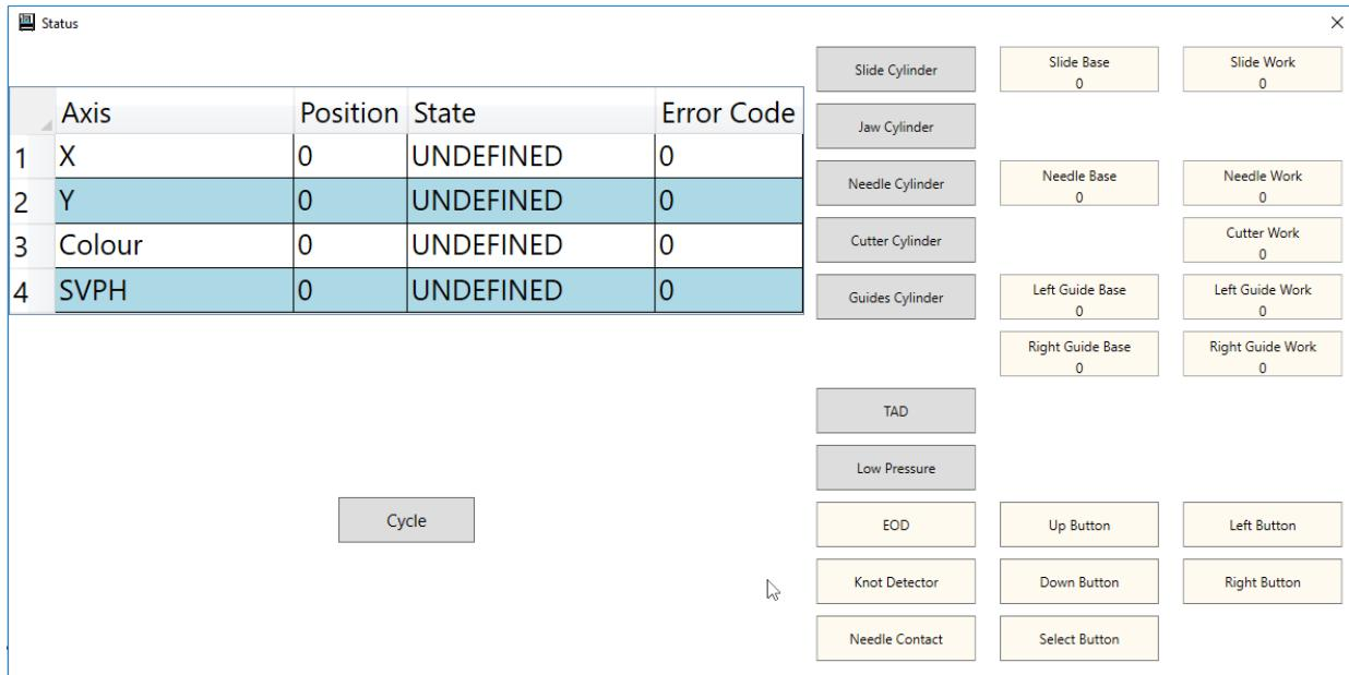
This screen enables the operator to switch the outputs **ON** and **OFF** for Kirby machine and reports the status of the inputs. This assists in determination of any Output or Input related problem and assists in the adjustment of cylinder limit switches. The numbers represent how long it takes for the action to be performed in milliseconds, this is used for diagnostic purposes.
