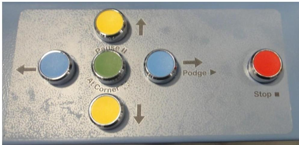
Select the **LEFT**, **RIGHT**, **UP** and **DOWN** buttons on the button panel to move the head and pegboard so that the needle can be manually inserted into the correct corner hole on the pegboard without it touching the sides of the hole. If the needle is touching the board, a message will appear on the screen "Needle Touching Board".
