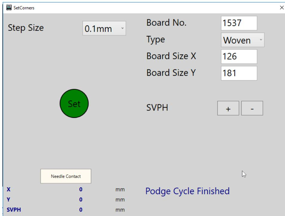
The *Corner Set* function is used to locate the exact positions of the 4 corner holes of each pegboard to be used on the machine.
